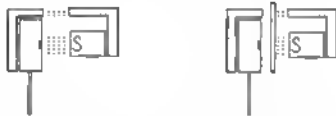
Fig.167 shows an arrangement for a concentrator. The concentrator allows the use of less powerful magnets or greater separation. Direct magnetic influence or a vane can still be used.
